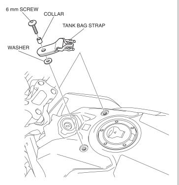
7. Install the tank bag on the fuel tank as shown.
